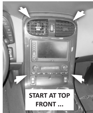
68. Starting at the front of the front console and working down and rearward, reattach it to the dash and console base.
