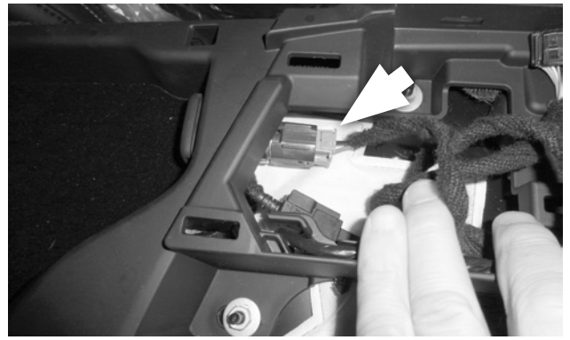
116. Reconnect the 12v power plug, and check the security of the connection.
